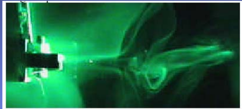
Fluid flow visualization from piezoelectric fan
