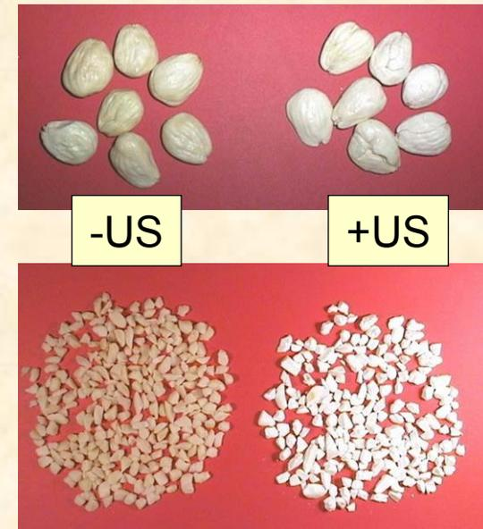
**At the end of the extraction time (after 8.5 hours) the loss of oil from the almonds was about 30% higher with US (50W at 20kHz).**
