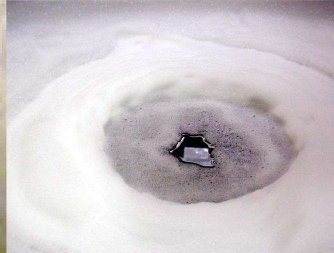
**FOAM BREAK IN THE CENTER OF THE REACTOR**
