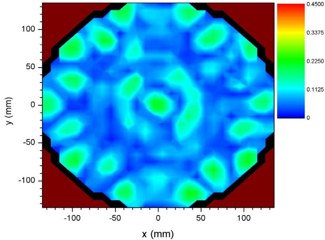
$V_{\text{rms}}(x,y)$  at 500W ( $dx = dy = 10\text{mm}$ , 25.6 - 33.9 °C, colour ranges: 0.1 - 0.45).
