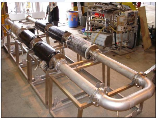
Flow through 10 bar, 70°C, 6M NaOH
