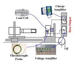
Figure 1: Diagram of the ultrasonic cutting rig used for cutting under constant applied loads
