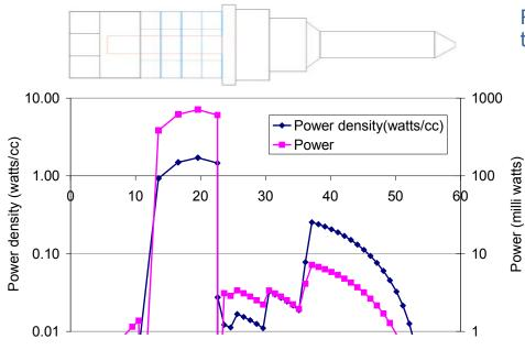
Relates to a maximum safe power condition where the stack temperature is limited to 60 °C
