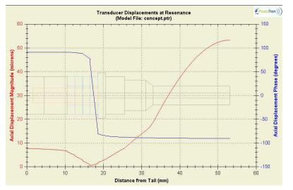
Cyclic stress in aluminum horn limited to 200 MPa p-p
