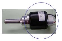
40 kHz test transducer with Stainless steel end masses
