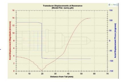
For an aluminum horn the ratio of the horn step stress to the max. piezo stress should be approximately 4.4 : 1.
