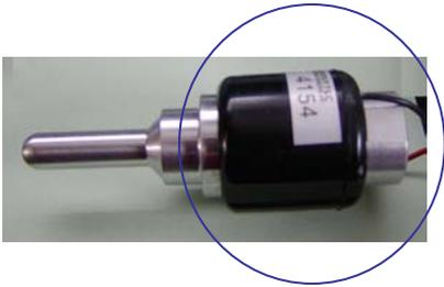
40 kHz test transducer with Stainless steel end masses
