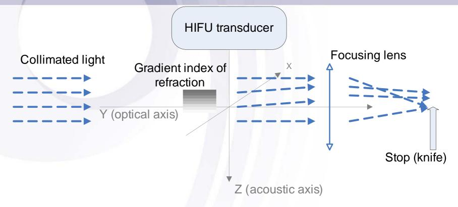
Spatial pressure gradients induce gradients in index of refraction All the parallel light impinges on the stop Only the deflected light passes the stop
