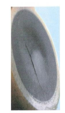
FIGURE 1. Cracked transducer front face due to an excessive applied power (about twice the maximal acceptable excitation level)
