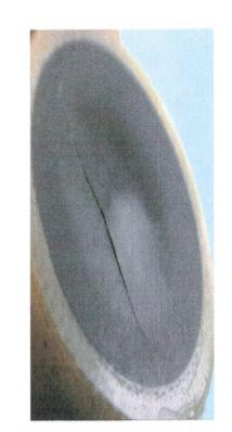
FIGURE 1. Cracked transducer front face due to an excessive applied power (about twice the maximal acceptable excitation level)
