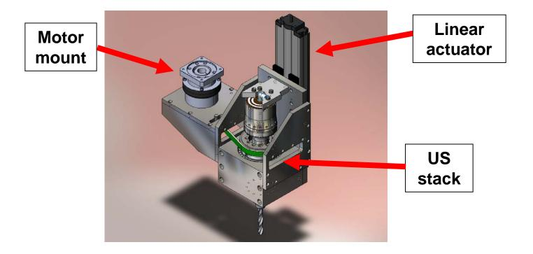
Drill head design: Mounts on standard "knee" mill
