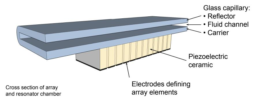
Resonance frequency: 2.5 MHz Channel thickness: 300 µm Reflector thickness: 300 µm Transducer thickness: 1 mm Element pitch: 500 µm
