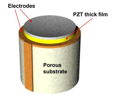
Typical structure of a thick film based HF acoustic transducer
