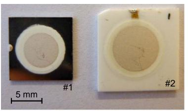
KNN-based thick films printed on silicon (#1) and alumina (#2) substrates.
