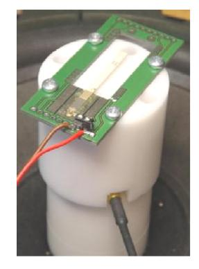
Energy harvesting device mounted on the shaker
