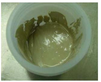
Fabricated piezoelectric paste
