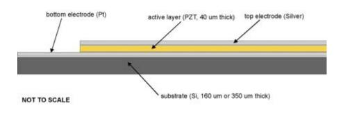
Structure of the thick film based silicon actuator/bender
