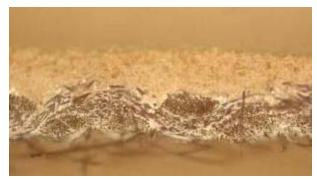
Cross section: Thick film on fabric
