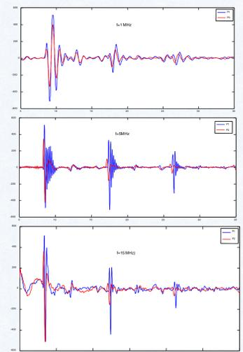
Fig. 1. Echoes in 3 points of the coarse-grained steel piece, with 3 transducers
