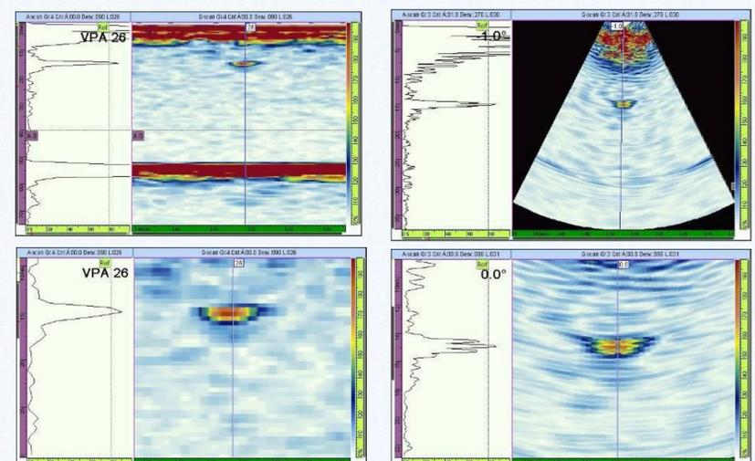
Fig. 2. Some array inspection results with Omniscan for an artificial flaw
